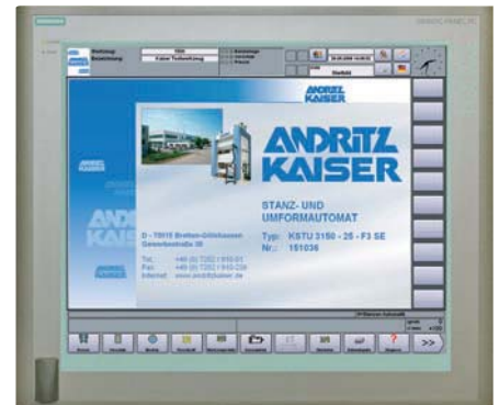
Andritz Kaiser PC Control SIMATIC S7-300 with PC 677 touch and 19" TFT colour monitor (option)
