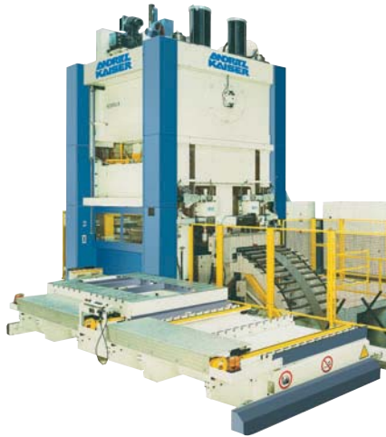
KSTU 6300-30-8 G RK with automatic retooling device
